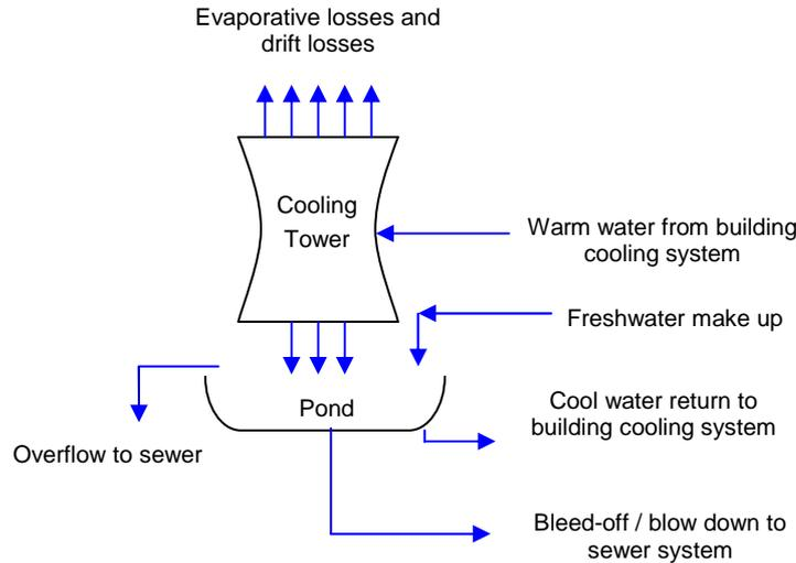
The losses from a cooling system which incorporates one or more cooling towers comprise leaks from the reticulation network, evaporation from the cooling tower itself, cooling tower overflows, drift losses and blow down (also called bleed-off) of concentrated cooling water. The sum of these losses is equal to the total volume of make-up water required to maintain the volume in the cooling system. This is represented by the simple mass-balance relationship:
